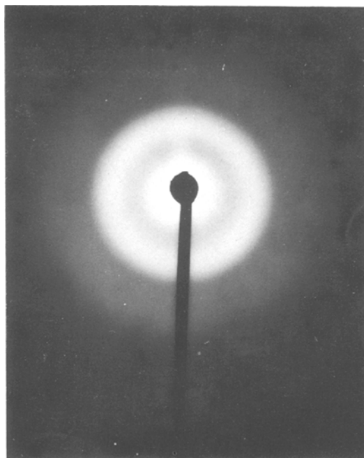
Figure 3 Diffraction pattern from a hydrate gel coating formed by dipping a thinned clinker into water.
