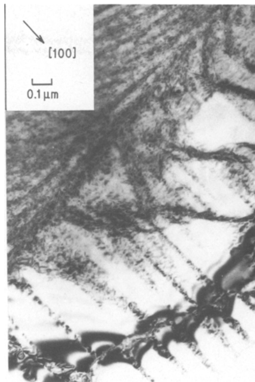
Figure 8 Precipitates in tricalcium aluminate.
